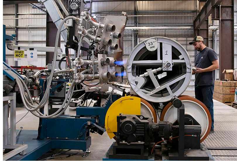
A Krah staff member checks the temperature of a pipe mandrel to make sure it is ready for hot strips of polyethylene to be wrapped around it.
